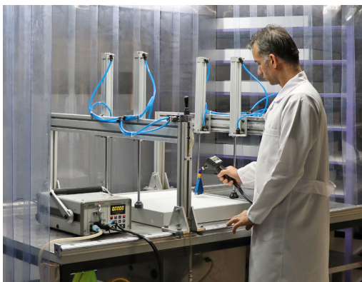
HEPA / ULPA Filter Test System - HF-SCAN 3004
