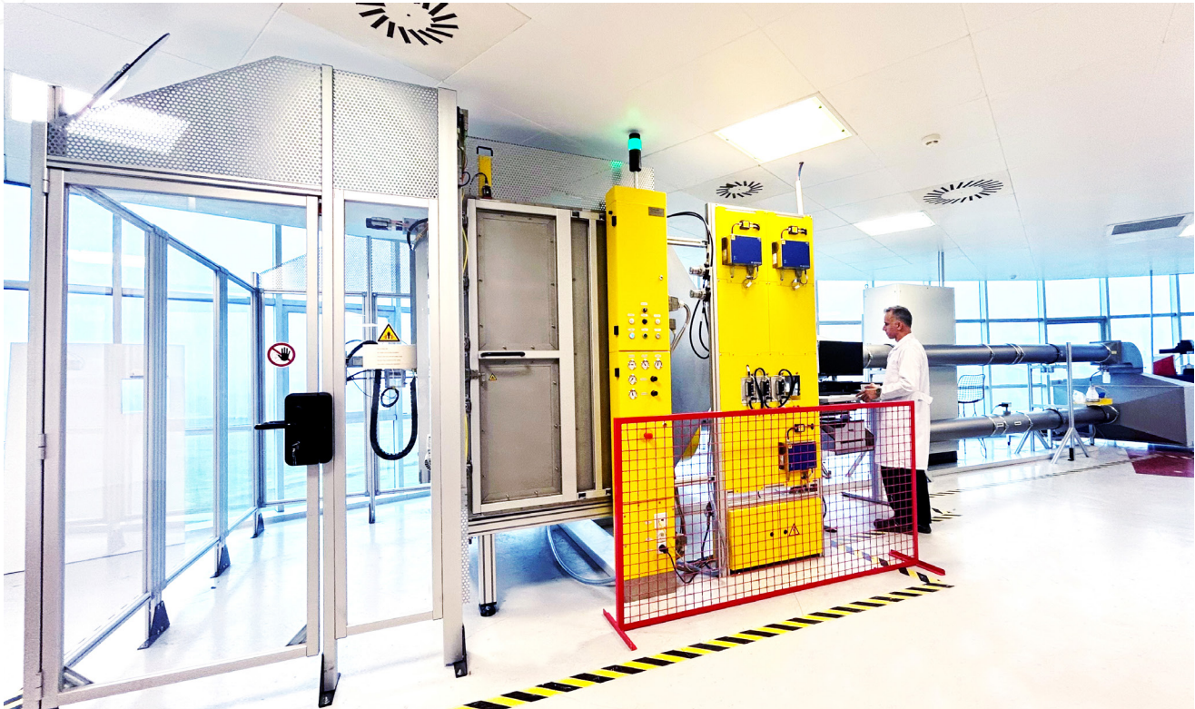
HEPA / ULPA Filter Test System - HF-SCAN 4002/2
